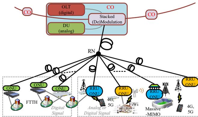
Fig. 1. Schematic architecture supporting FMC by using the proposed stacked modulation scheme.
