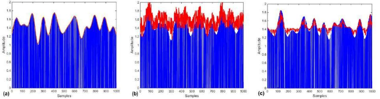
Fig. 6. Envelope detection with (a) image edge detection, (b) bandpass FIR filter and (c) Hilbert transform method. (the original stacked modulated signal (blue curve) and the one detected by different methods (red curve))
