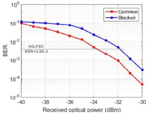
Fig. 8. BER versus optical received power of OOK.
