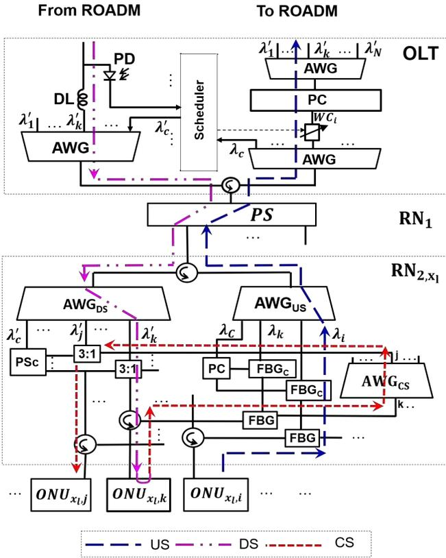
Fig. 1. Proposed Architecture for OLT and Remote Nodes. PC- Power Combiner, 3:1- 3:1 PC, DL- Delay Line, PD- Photo Detector
