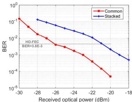
Fig. 9. BER versus optical received power of OFDM.
