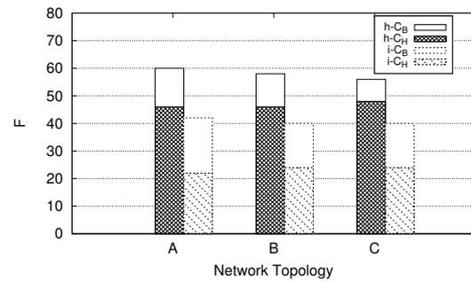
Fig. 5. Total cost  $F$ , normalized with respect to  $\alpha$ , for ILP (i) and heuristic (h), representing the contributions of the BBU hotel activation cost  $C_B$  and the overall distance between each pair of RRUs and BBU hotels  $C_H$ , in networks A, B and C when  $R = 2$ .
