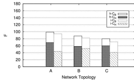
Fig. 6. Total cost  $F$ , normalized with respect to  $\alpha$ , for ILP (i) and heuristic (h), representing the contributions of the BBU hotel activation cost  $C_B$  and the overall distance between each pair of RRUs and BBU hotels  $C_H$ , in networks A, B and C when  $R = 10$ .
