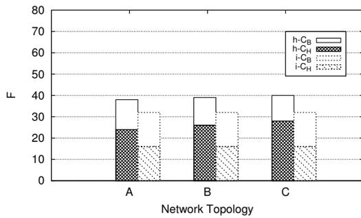
Fig. 4. Total cost  $F$ , normalized with respect to  $\alpha$ , for ILP (i) and heuristic (h), representing the contributions of the BBU hotel activation cost  $C_B$  and the overall distance between each pair of RRUs and BBU hotels  $C_H$ , in networks A, B and C when  $R = 1$ .
