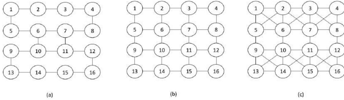
Fig. 3. The reference network topologies, (a) network A with connectivity  $N_A = 2.25$ , (b) network B with connectivity  $N_B = 3$  and (c) network C with connectivity  $N_C = 4.5$ .
