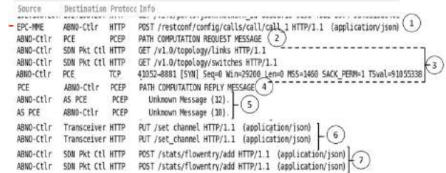
Fig. 4. Captured set of control messages exchanged between EPC and ABNO.
