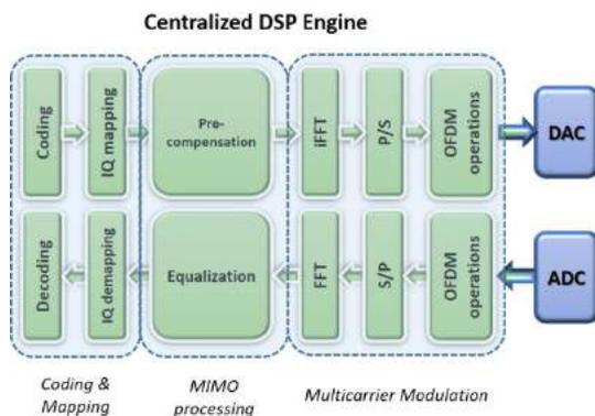
Figure 3: Centralized DSP engine for 5G-compatible Analog MFH.
