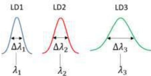
Fig. 2 The frequency domain of laser diodes pulses
