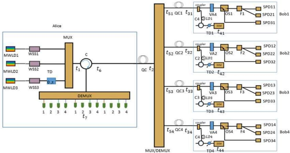
Fig. 1 Schematic of multi-user WDM-FT QKD system
