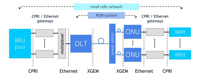
Lowest latencies achievable by fixed bandwidth assignment on the TDM-PON network
